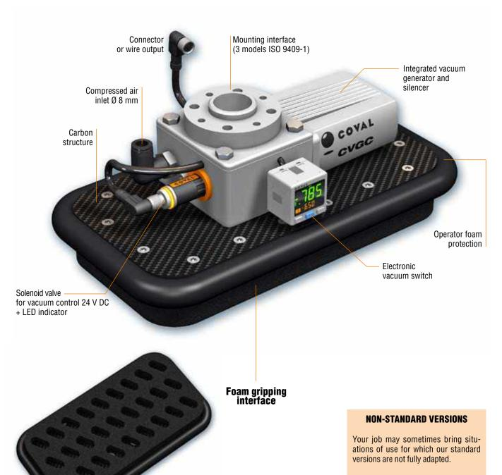
Coval is able to offer customized solutions by providing tailor-made vacuum grippers - adjustment of dimension or selection of gripping interface.
